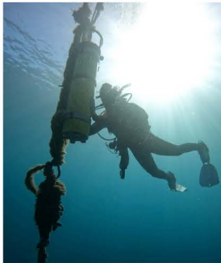
Below: Diver services an IFCB that detects phytoplankton and HAB blooms in real-time.
