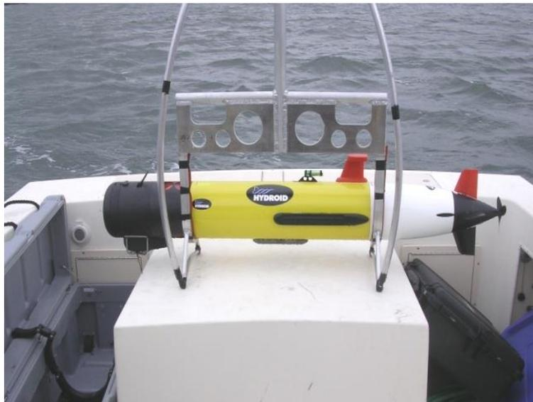
**Figure 8. REMUS AUV Mission used in OCSD diversion.**
