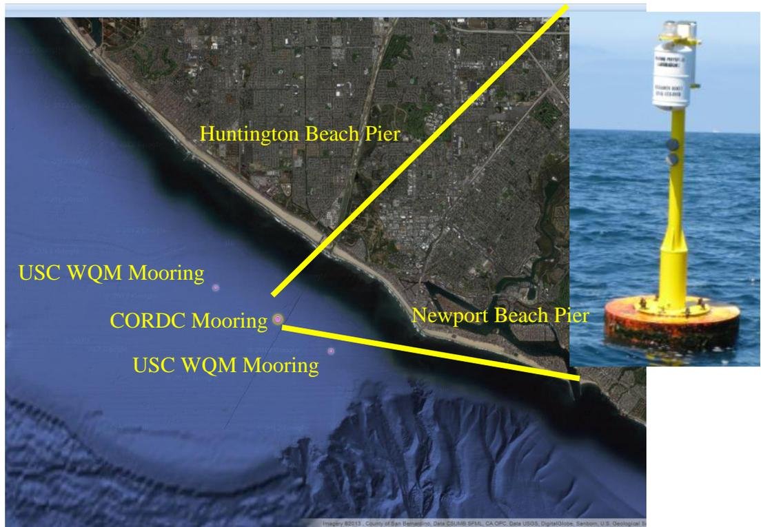
**Figure 2. CORDC and USC Mooring locations. The white cylinder on the mooring to the right is a radar reflector and the cylinder on the left is a GPS tracking device.**
