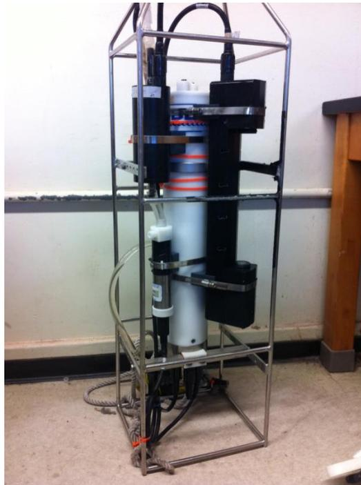
**Figure 7. Picture of CTD system used for sampling. White cylindrical instrument in center is CTD, small black cylindrical instrument (upper left) is CDOM fluorometer, and black instrument on right is transmissometer. Lab bench to right of instrument (shown for scale) is roughly 30 inches in height.**
